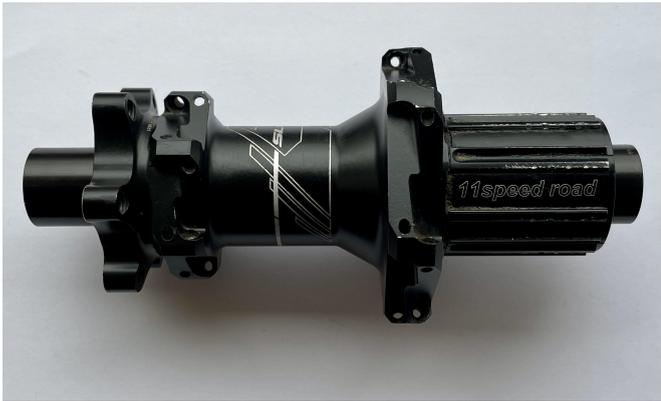
A black rear hub with a cassette attached. The cassette has "11speed road" printed on it. The hub has a silver logo on the side.  | <p>1</p> <p>Remove the cassette from the rear hub</p>                                                                         |
