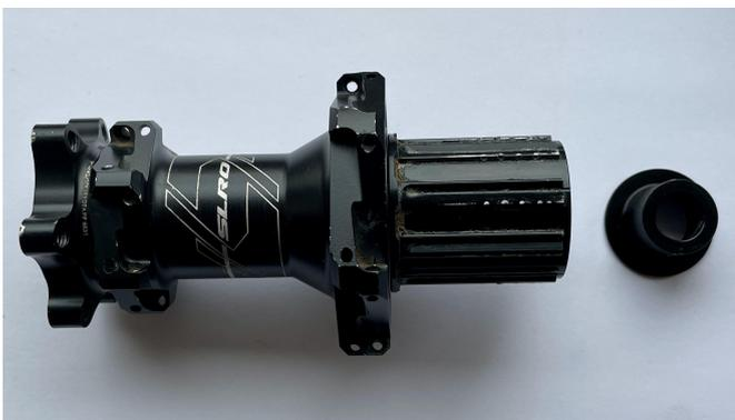
A rear hub is shown on a white surface with the end cap removed and placed to the right. The hub has a silver logo on the side. | <p>4</p> <p>Use a 5mm allen key and synthetic hammer to punch out opposing adapter, or alternatively use the vice again</p>   |
