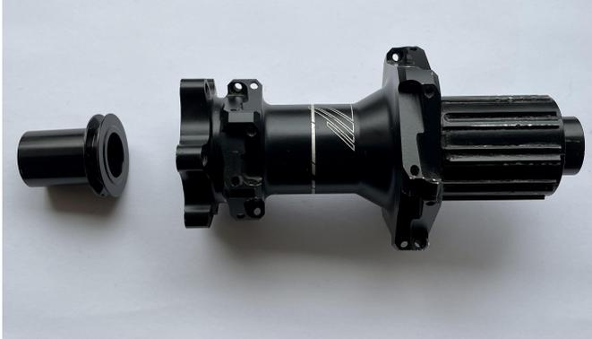
A rear hub and a black end cap are shown on a white surface. The end cap is a small, cylindrical component with a flange.       | <p>3</p> <p>Pull up on wheel to remove the adapter</p>                                                                        |
