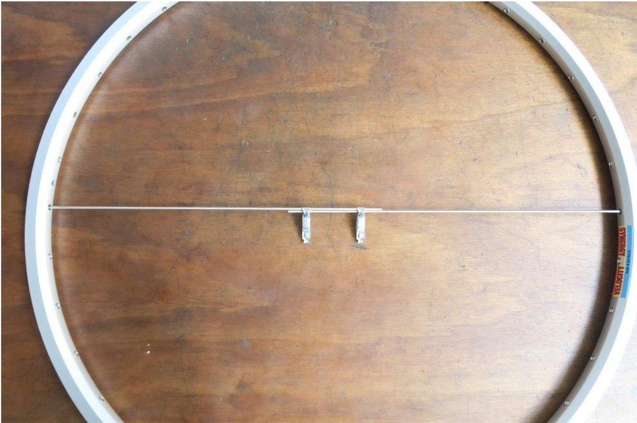
*The BSC ERD Rim Rods shown correctly placed into the rim.*
